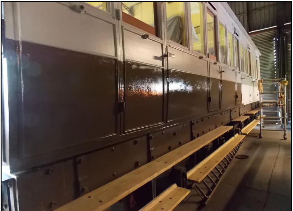
No.946 in grey primer (above) and receiving its first coats of brown and grey (below). photos: Clyde Pennington
